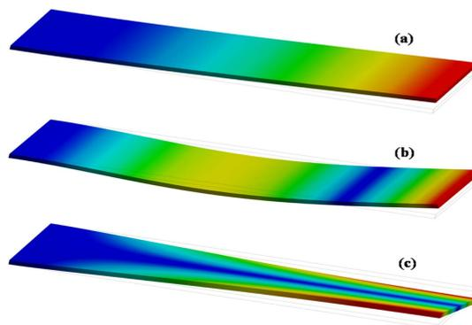
**Fig. 5.** Mode shapes for (a) mode 1 (b) mode 2 (c) mode 3 of 0.2 wt% GO incorporated CF/epoxy composite
