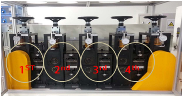
Fig. 6. 4 section of double belt laminator
