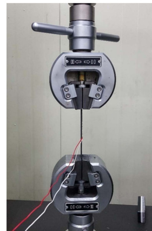
Fig. 3. Tensile test procedure of braided carbon/epoxy composites
