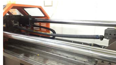
Fig. 16. Test process of compression test for TIE ROD
