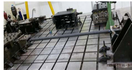
Fig. 17. Test process of Fatigue test for TIE ROD
