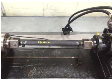
Fig. 14. Test process of tensile test for ball joint region
