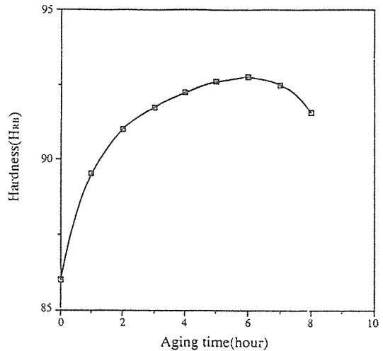
Fig. 7. Effect of aging time for Al/Al 2 O 3 (15%) composites
