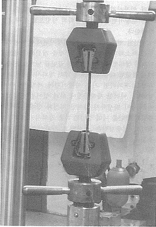
Fig. 4. The test set-up of original and modified tensile coupon specimens for tensile strength measurement.
