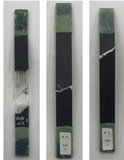
Fig. 7. Failure mode of G.O. (HSHT glass + Onyx)
