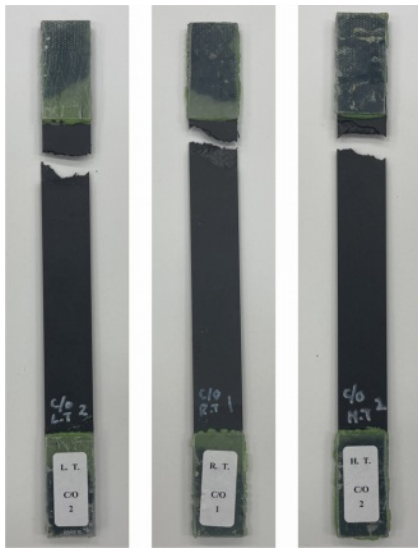
Fig. 5. Failure mode of C.O. (Carbon + Onyx)
