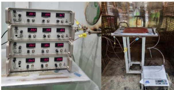
Fig. 5. Dielectric sensor and 4-channel cure monitoring system
