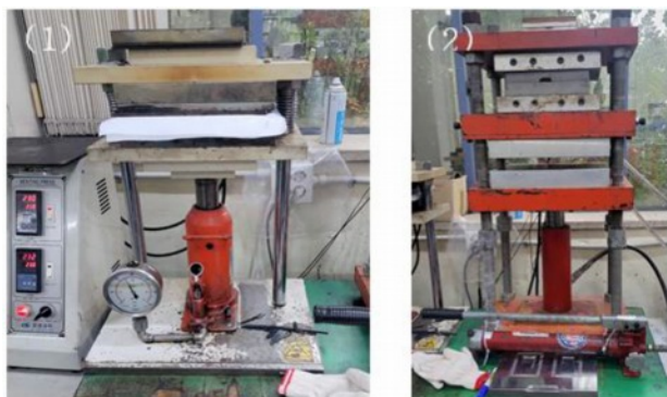
Fig. 1. Equipment used to produce carbon fiber reinforced composite materials; (1) Hot press, (2) Cooling press
