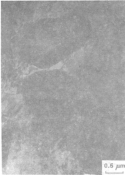
Fig. 8 Transmission electron micrograph of the 2124-T6 aluminum matrix composite reinforced with 13.2 v/o SiCw.
