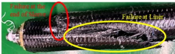
Fig. 14. Burst pressure test result of baseline design
