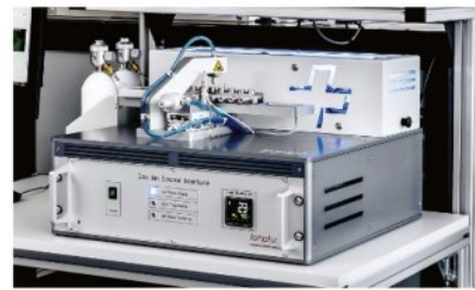
(b) The gas interface system for AMS [14]
