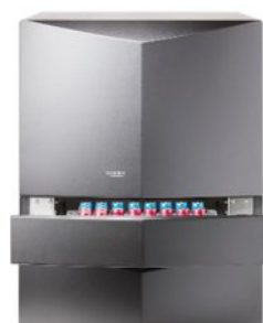
Fig. 1. Low-level liquid scintillation counter [6]
