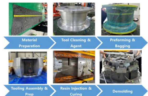
Fig. 7. Duct manufacturing process
