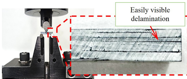
Fig. 15. Failure mode by interlaminar shear test
