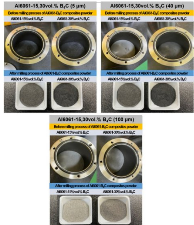
Fig. 1. B_4C -Al6061 powders mixed with different B_4C particles
