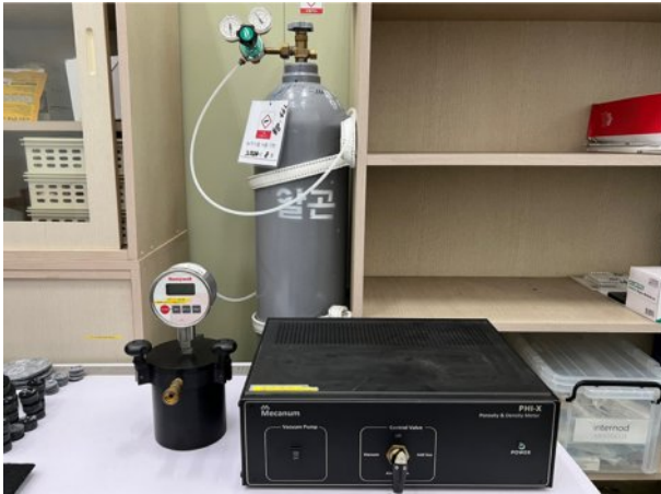
Fig. 11. Phi-X and SIGMA-X system used to measure porosity, flow resistivity, and other acoustic parameters
