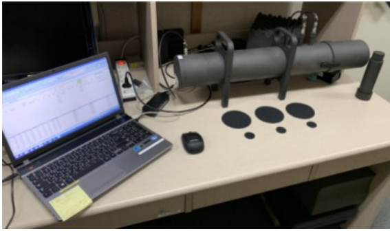
Fig. 5. Acoustic impedance tube setup (Scien 9301) for low- and high-frequency absorption measurements based on KS F 2814-2
