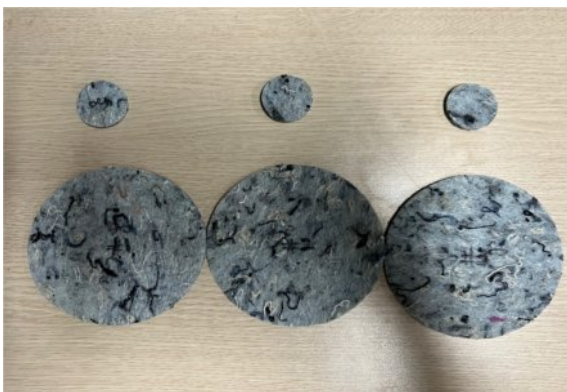
Fig. 6. Preparation of circular test specimens (Ø100 mm and Ø29 mm) for low- and high-frequency impedance tube testing
