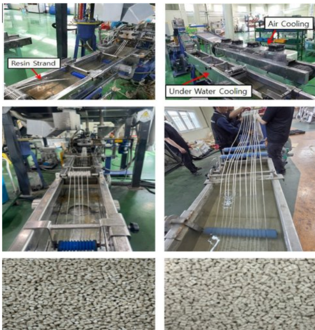
Fig. 6. Scale-up Process and Equipment Transition from 32 mm (L) to 48 mm(R) Twin-Screw Extruder
