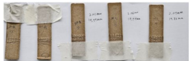
Fig. 5. Deformation of molded pulp specimen during in-plane compression test showing suppressed global buckling
