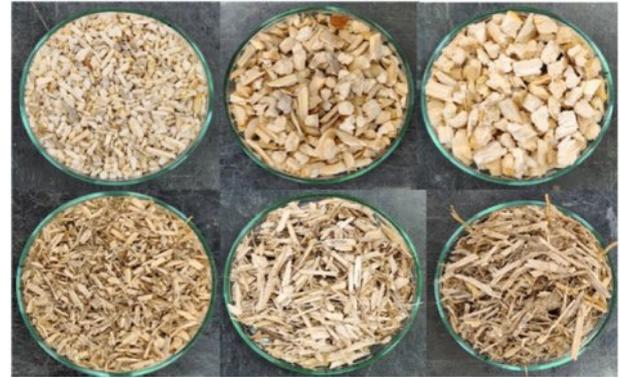
Fig. 1. Photographs of hemp and kenaf hurds (Top: Kenaf, Bottom: Hemp, From left to right: Core sizes 3, 5, and 8 mm)
