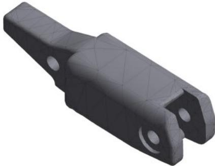
Fig. 2. Finite element mesh of a single chain link
