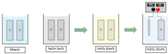
Fig. 1. Schematic illustration of the anodizing process for aluminum surface treatment
