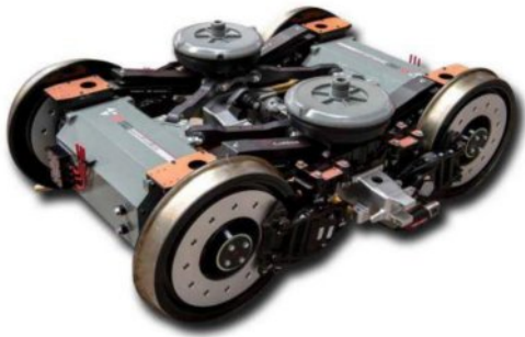
Fig. 13. Acro bogie featuring carbon fiber composite side beams
