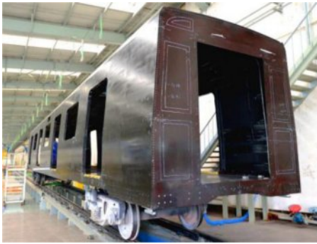
Fig. 8. Carbon composite body of CETROVO 1.0 train
