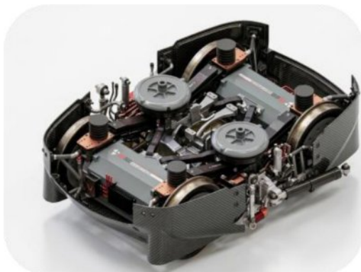
Fig. 16. Composite material bogie cover installed on the bogie
