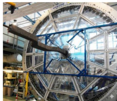
Fig. 18. Side beam fabrication through the braiding process
