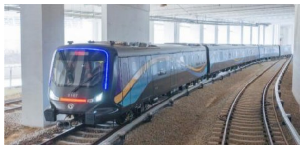
Fig. 7. Urban train with composite body(CETROVO 1.0)
