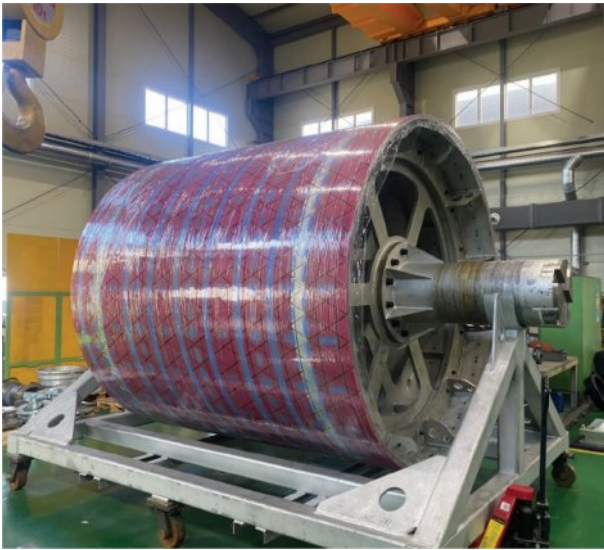
Fig. 17. Manufacturing of Cylindrical Lattice Structure(2)
