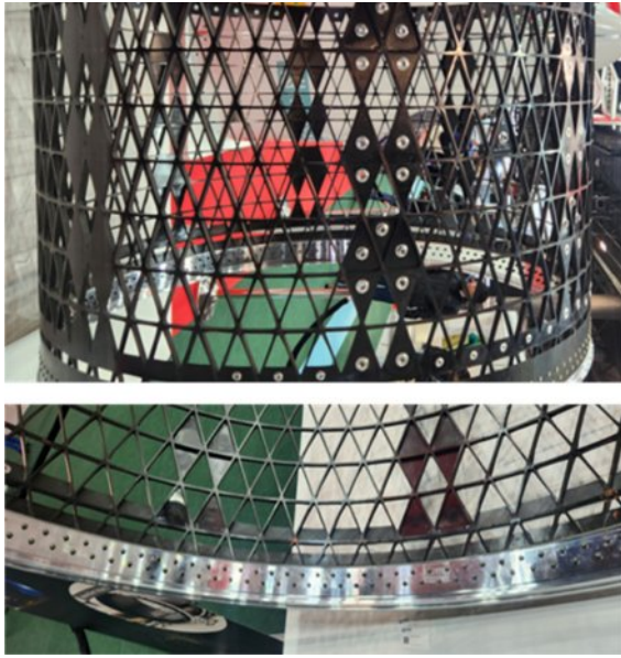
Fig. 25. Application Interface on Lattice Structure
