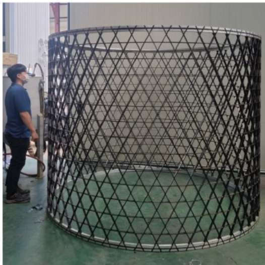
Fig. 18. Manufacturing of Cylindrical Lattice Structure(3)
