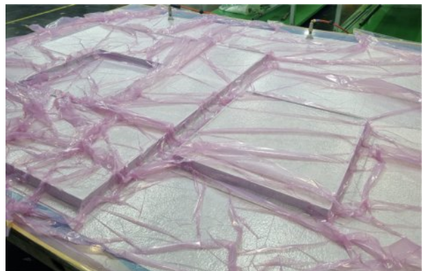
Fig. 11. Manufacturing of Sandwich Panel Structure(2)
