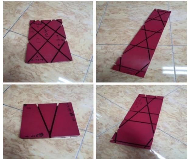
Fig. 15. Manufacturing mould for Lattice Structure
