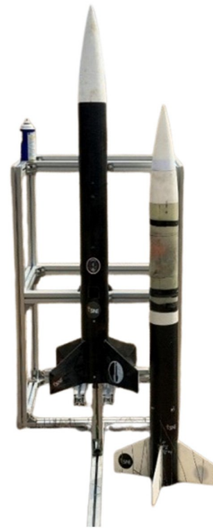
Fig. 8. Completed LW-PLA model rocket (total length: 1200 mm, maximum outer diameter: 104 mm)
