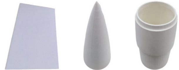
Fig. 3. Rocket components (nose cone and fins) fabricated from LW-PLA
