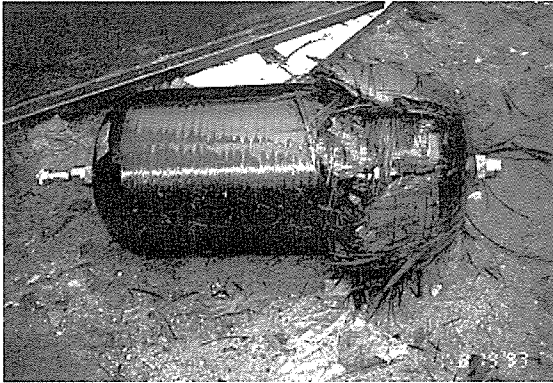
Fig. 13 A picture of fractured vessel.
