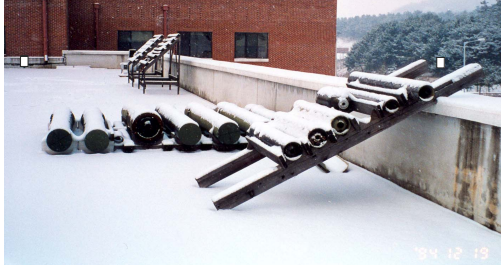
Fig. 3 Natural aging test at outdoor.
