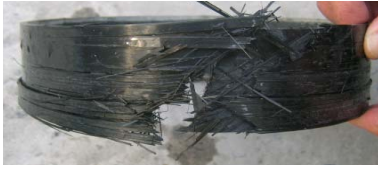
Fig. 6 Hoop ring specimen after failure.
