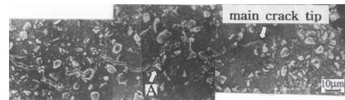
(b) N=6.63\times 10^4 cycles, 2a=2.05 , K_{\max}=6.53\text{MPa m}^{1/2}
