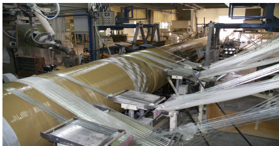
Fig. 1 Manufacturing process of GFRP Pipe(Hankuk Fiber Co.[1]).
