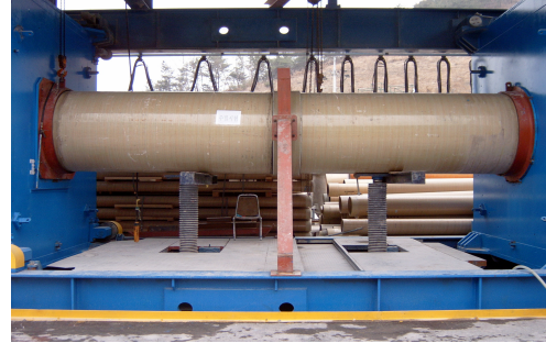
Fig. 14 Watertightness test at the joint.
