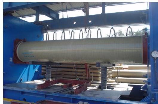
Fig. 11 Water pressure test of GFRP pipe.
