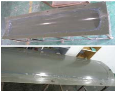
Fig. 8 Preparation of Mold.
