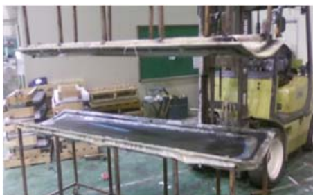
Fig. 11 Assembly of Upper mold and Lower mold.
