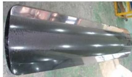
Fig. 13 Completed Composite Cradle.
