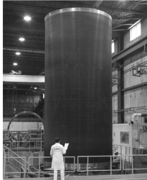
Fig. 3 Space shuttle's filament wound case segment.
