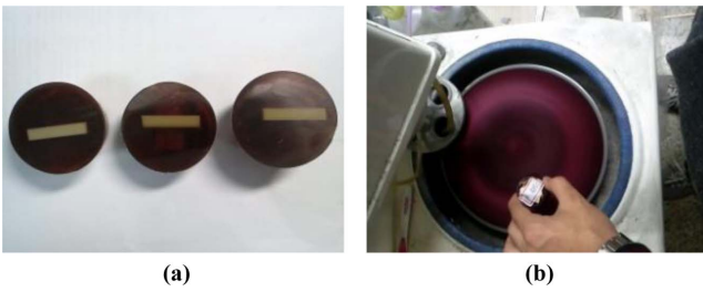
Fig. 5. (a) Microscopic image specimen (b) Polishing process.
