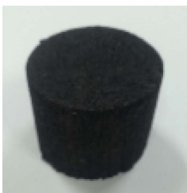
Fig. 1. Foam specimen of EPP
