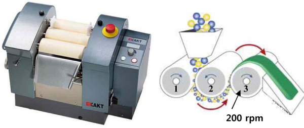
Fig. 1. Three-roll-mill (dispersion equipment)
