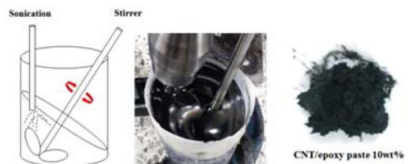
Fig. 1. Manufacturing process of 10 wt% CNT paste
