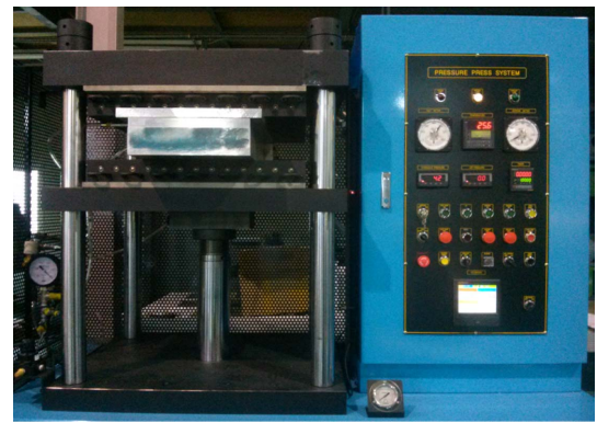
Fig. 2. Pressure press process equipment
