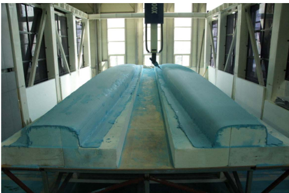
(a) Hull/Deck Plug Mold Using 5-Axis Machine
