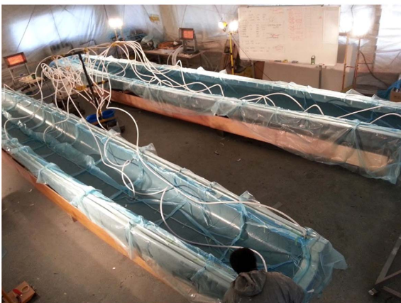
(b) Vacuum Infusion Method of Construction
